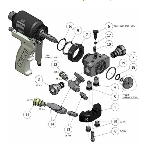
Figure 2. Ball Valve Final Assembly (OPTIONAL)
