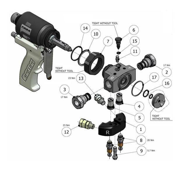
Figure 1. Standard Final Assembly, Master III Gun
