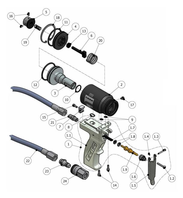
Figure 3. Air Cylinder and Grip Assembly
