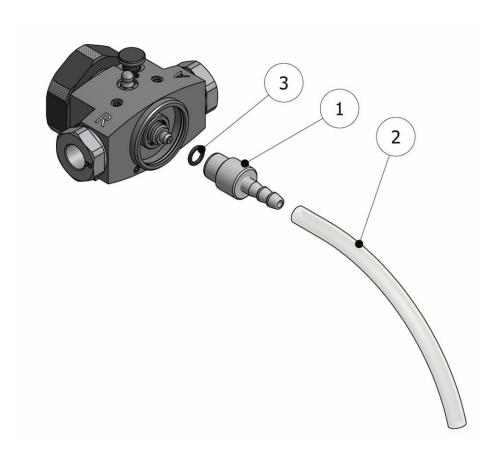
Figure 9. Assembly Pour Adapter (OPTIONAL)
