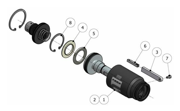
Figure 4. Magnetic Micro Assembly (OPTIONAL)
