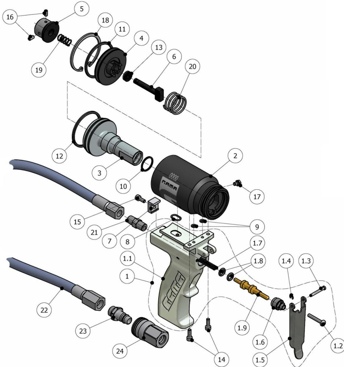
Figure 3. Air Cylinder and Grip Assembly
