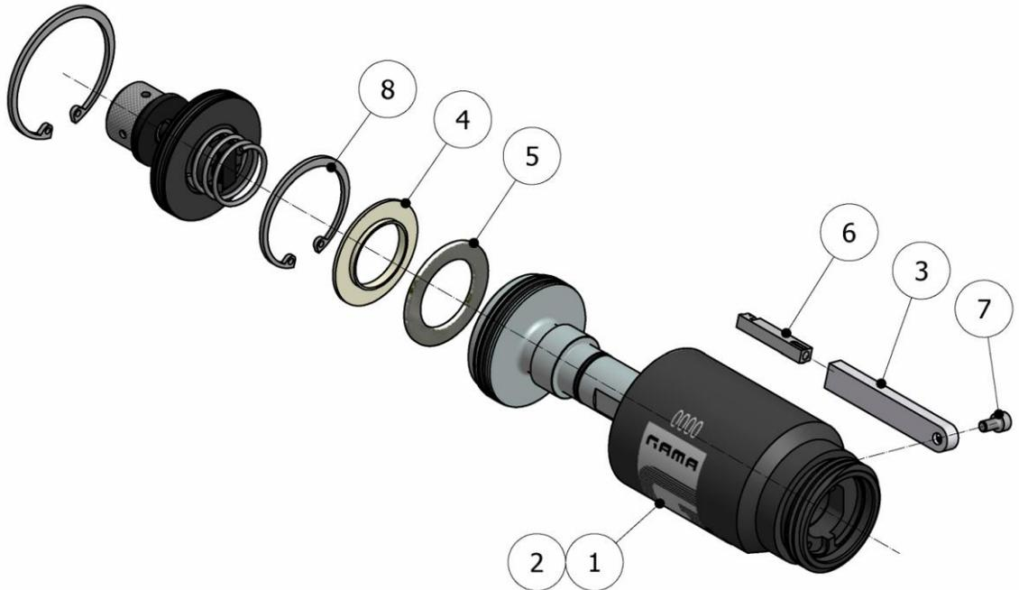
Figure 4. Magnetic Micro Assembly (OPTIONAL)
