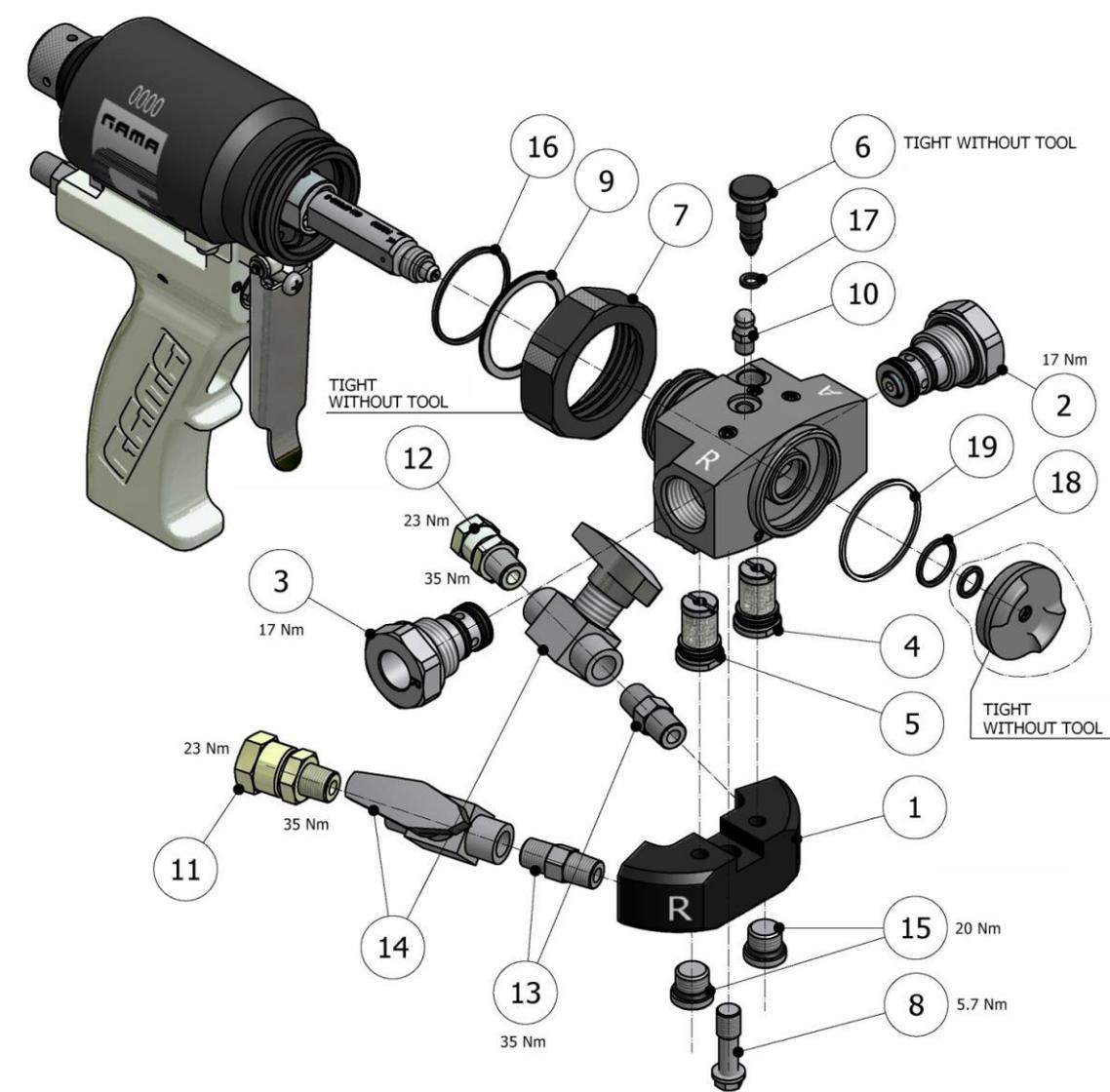
**Figure 2. Ball Valve Final Assembly (OPTIONAL)
