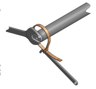
Use a belt spanner (not supplied) to loosen the valve, if necessary, placing it as close as possible to the end of the pipe in order to avoid deformations.
