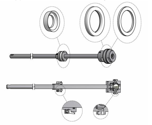
9. Lubricate and fit all parts in reverse order to the process described above.
