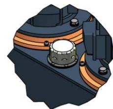
**NB:** Do not fill the tank to maximum capacity (128 Lts – 34 gal); make sure the amount of oil is not more than 80% of its maximum capacity (100 Lts. – 26 gal). Use the visual level indicator of temperature on the tank as a reference, because the maximum temperature limit (80°C – 176°F) coincides with the advised capacity.
