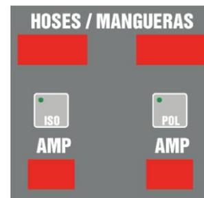
The push-buttons turn on or off the hose heating system of each product. Each push-button has a led that lights when the heater is on; if the led flashes, it indicates that the system is not heating; if the led lights steady, it indicates that the system is heating.
