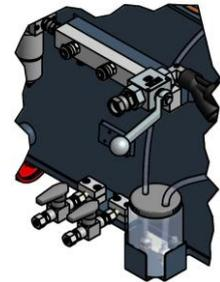
**CAUTION!** *To avoid excessive pressure in the heating hoses, wait for the product in them to reach the required temperature before starting up the hydraulic system.*
