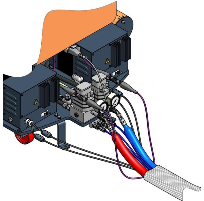
**NB:** To protect the TCS sensor, you must pay special attention not to kink or excessively bend the hoses. Do not roll up the hoses with a radius of under one meter / 3 feet.
