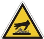
***The unit includes components that reach temperatures that are liable to cause burns. The hot parts of the unit must not be handled until they have cooled.***
