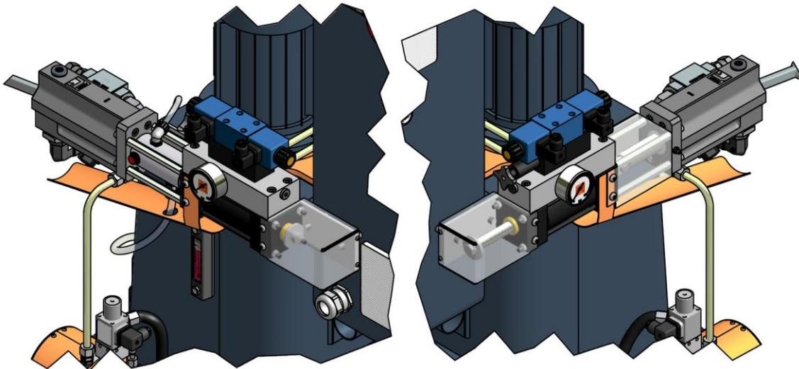
If excessive pressure is caused in the Isocyanate circuit or the Polyol circuit, an audible alarm will be activated, and the control panel will show the alarm screen ISO/POL HIGH PRESSURE.
