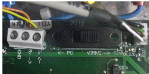
**NOTE:** The unit must be turned off to be able to work on the DIP selector.
