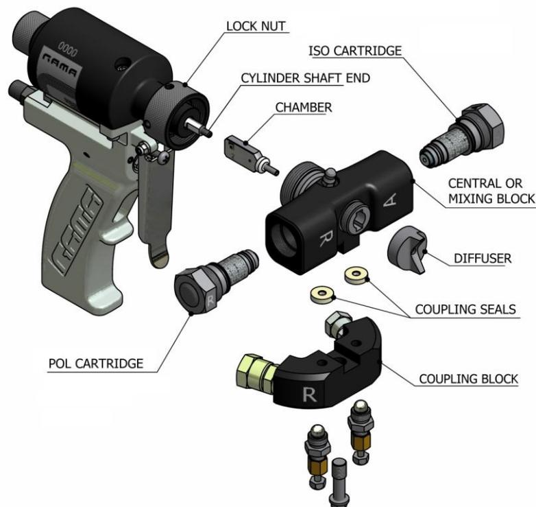
**PRECAUTION:** To avoid spilling the rest of the product which has accumulated in the side cartridges onto the floor, always remove the coupling block and the side cartridges on a waste vessel.
