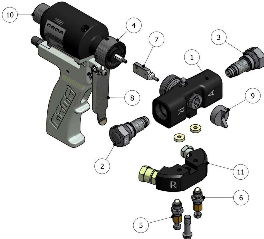
The main components and their description are given for better knowledge of the elements of the **MASTER II** series gun. For more precise identification, see the Components Manual ref. NR-00020-ENG
