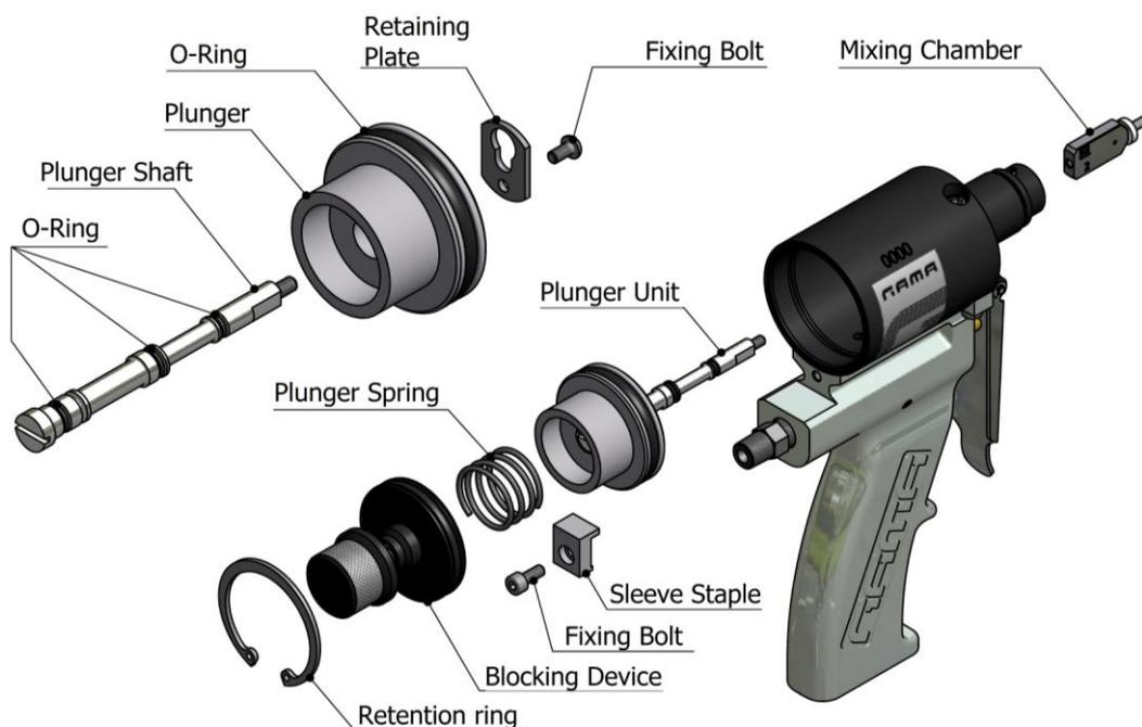
1. Proceed to remove the mix chamber following the procedure indicated in the **Gun block unit and mix chamber** section. Clean the mix chamber and, if necessary, redo the holes with a drill.
