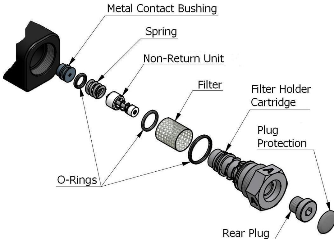
**PRECAUTION!** Use wooden or plastic utensils or a brass brush for cleaning. Do not use metal utensils, which can scratch the contact surfaces.
