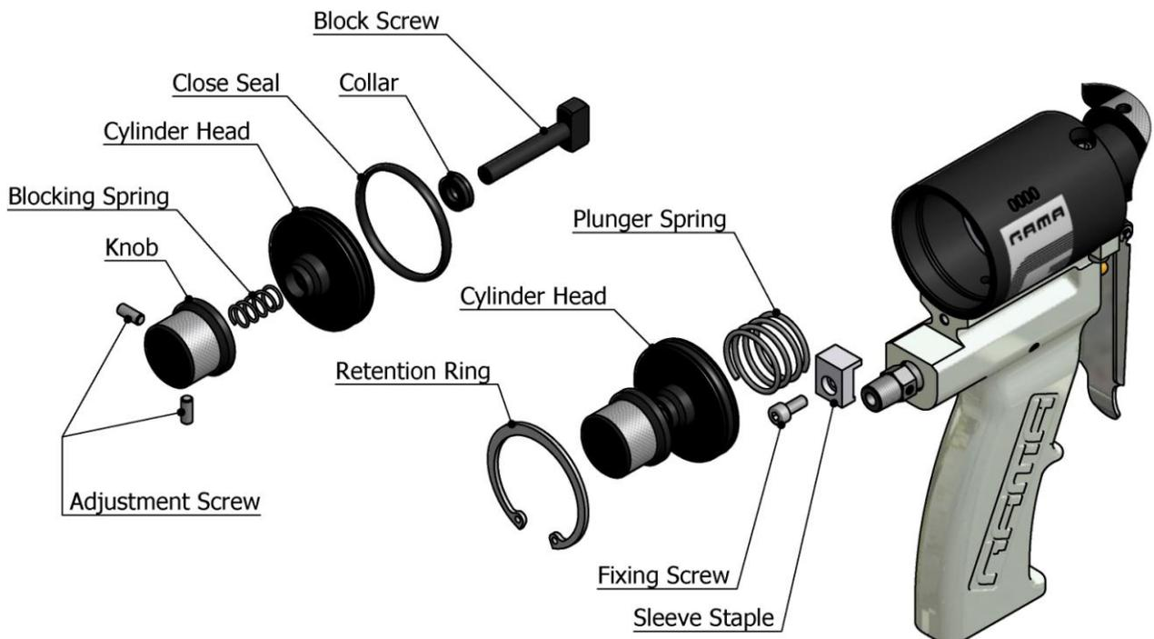
1. Unscrew the screw fixing the sleeve staple on the rear of the gun.
