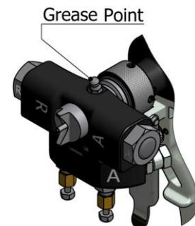
**NOTE:** The action of greasing the gun at the end of the day will avoid maintenance time, as it will not be necessary to dismantle the chamber each day to clean it.
