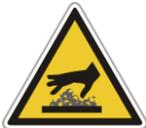
***The equipment includes components which reach high temperatures and may cause burns. The hot parts of the unit must not be handled or touched until they have completely cooled.***
