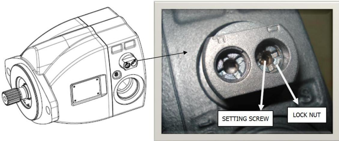
When the setting screw cannot be turned clockwise or counter clockwise easily, is because the lock nut is jammed up against the setting screw. In this case, turn clockwise the setting screw to unlock the lock nut.
