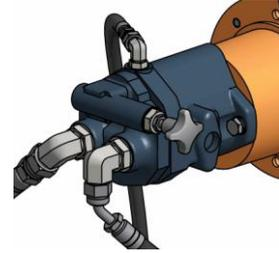
**With BR Pump.-** The pressure is set with the pressure setting screw (position D).
