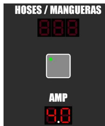
To select the temperature when the unit is working in automatic heating control mode, touch the MODE button, select the desired temperature using the UP/DOWN buttons and touch the MODE button again to confirm the setting. Follow the same procedure to select the amperage. When the unit is operating in automatic control mode, this value should be set to between 4.5 and 5.0 amps.
